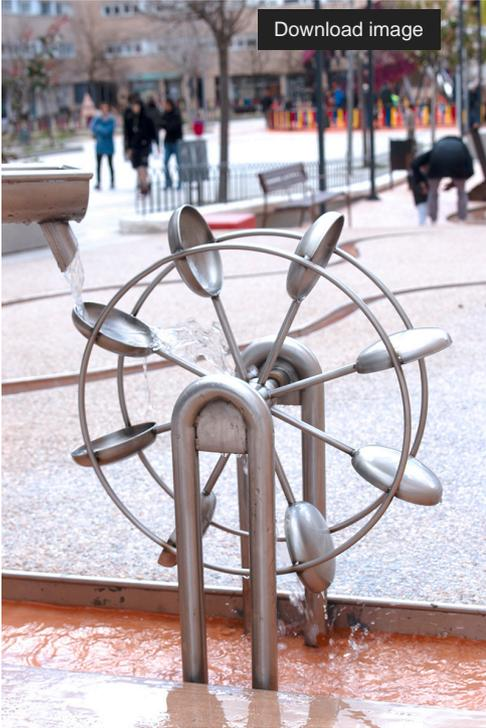
Playgrounds are often exposed to severe environmental conditions, such as rain, humidity and sun exposure. In their manufacture, it is preferred to use materials such as stainless steel, which is highly resistant to corrosion and maintains its structural integrity over time.
