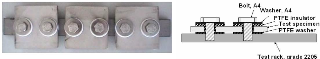
Figure 1. Test rack for mill exposure and coupon assembly.
