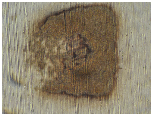
Figure 8.8: Example of experiment 6, P = 300mW and 15 pulses. No energy in the middle.
