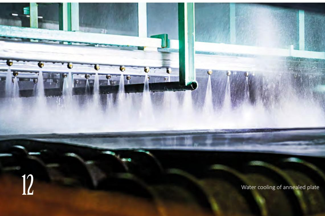
Water cooling of annealed plate
