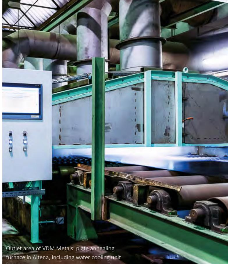
Outlet area of VDM Metals' plate annealing furnace in Altena, including water cooling unit
