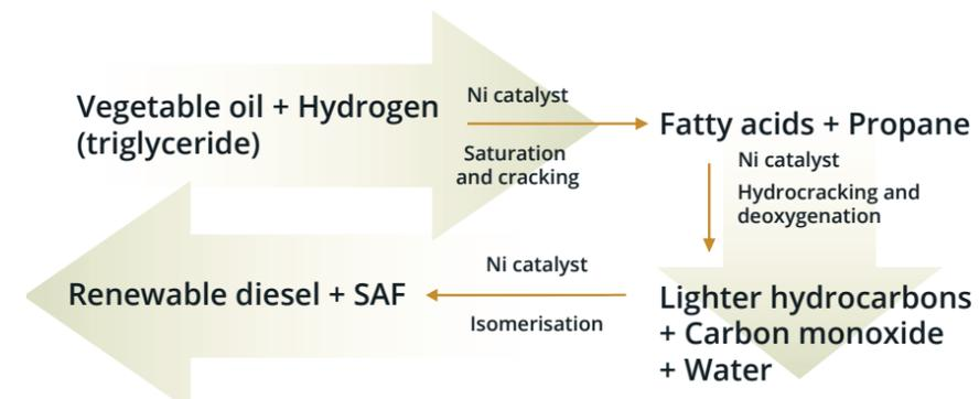
Figure 2. Chemical steps in the hydrotreating of vegetable oils to make renewable diesel.
