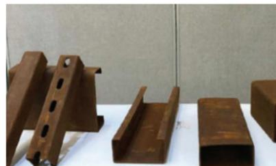
*Weathering steel components for solar photovoltaic racking systems*
