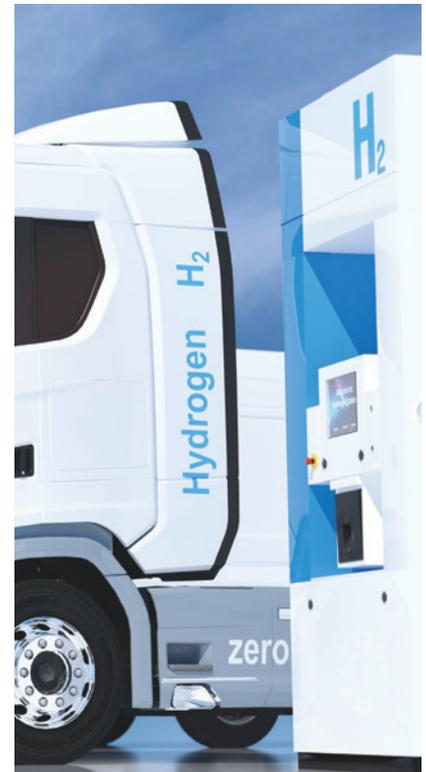
*Proton exchange membrane fuel cells (PEMFC) are the most widely used and commonly deployed in mobile applications such as cars, trucks, buses, and forklifts due to their size flexibility, favourable power-to-weight ratio, and fast start up.*
