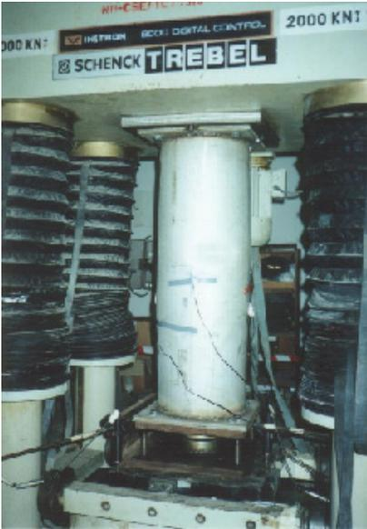
**Figure 4** Typical CHS column test
