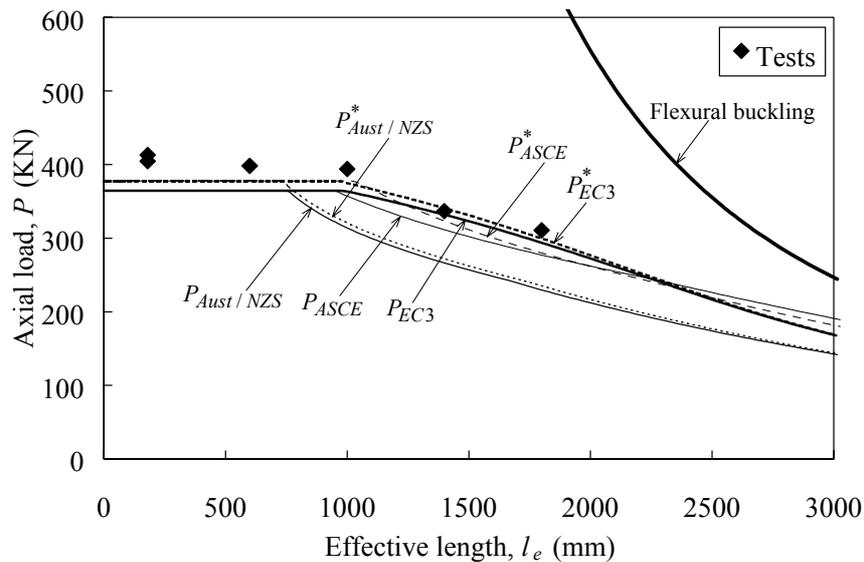
**Figure 3** Fixed-ended column curves for RHS Series R3
