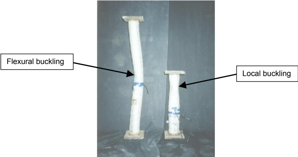
**Figure 5** Flexural buckling and local buckling of CHS columns
