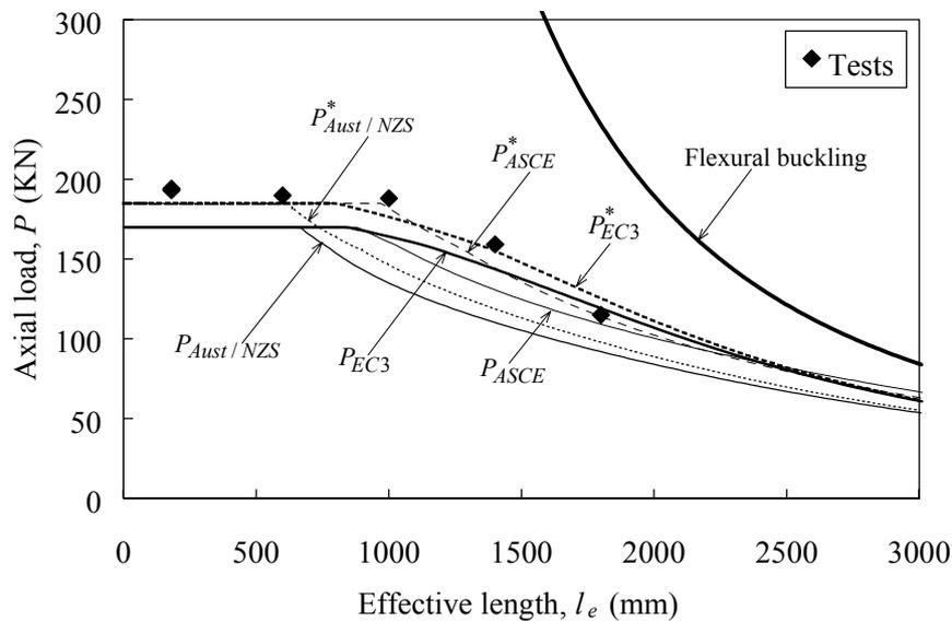
Figure 2 Fixed-ended column curves for SHS Series S1
