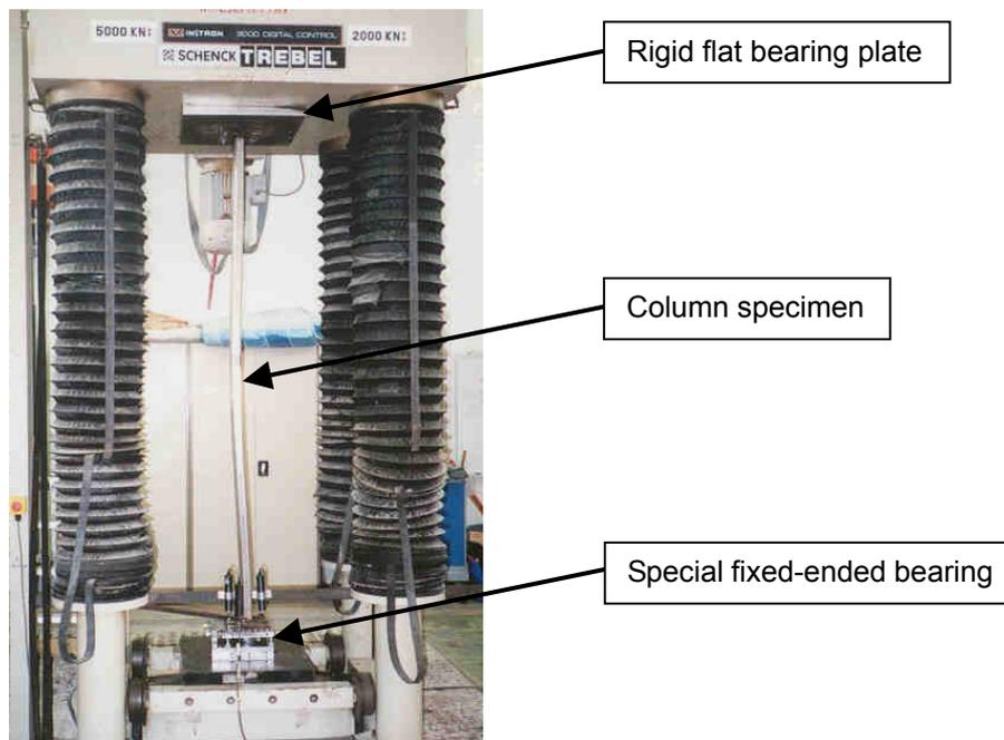
**Figure 1** Test set-up
