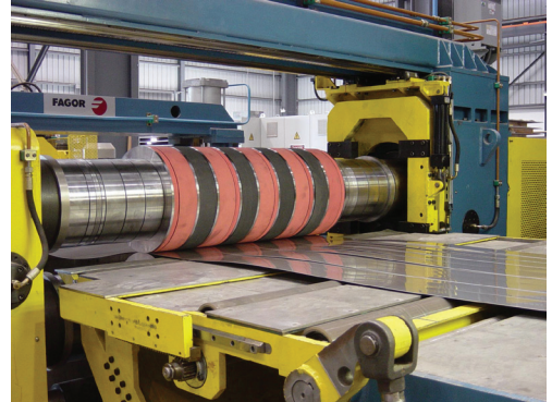
Photo 3: Slitting line in action
