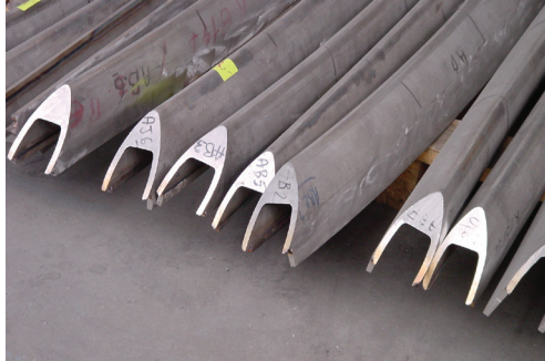
Photo 8: Hot extruded sections, used for the glass-steel structure “La lentille de la cour de Rome” (The lens of the Rome yard) – Paris (F)
