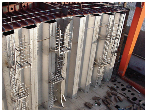
Photo 17: Duplex stainless steel bulkhead panels for chemical tankers
