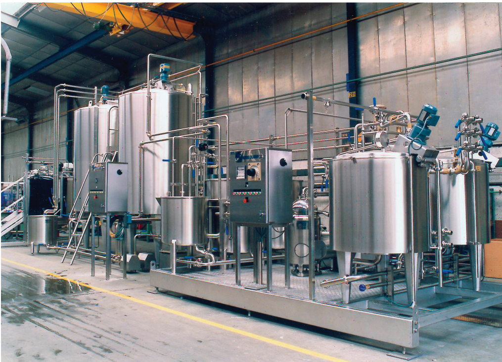
Photo 11: Milk pasteurizing plant
