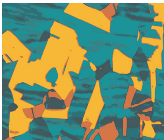
Fig. 1 - Austenitic stainless steel micro structure with austenite grains free of precipitates.
