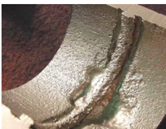
Fig. 2 - Stainless 304 pipe with intergranular corrosion in the heat affected zone
