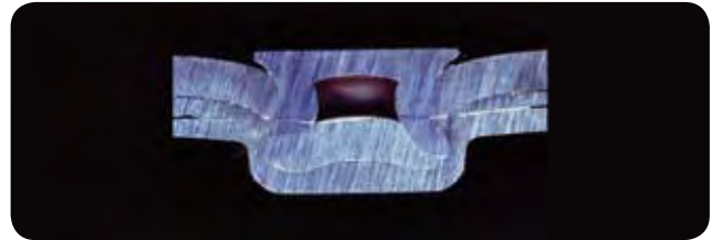
Auto-riveting on 430, 1.5 mm.
