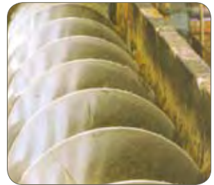
Grade 1.4003/410, Columbus, S. Africa. Here, ferritic has lasted over 18 years.
