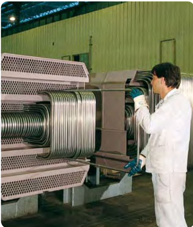
Moisture separator reheater in grade 439, Europe.
