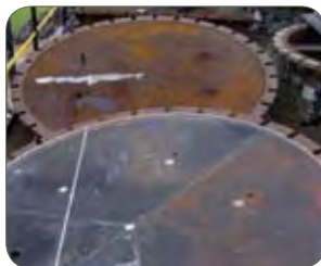
Grade 1.4003/410, Columbus, S. Africa. Carbon steel (top) compared to ferritic (bottom) after 6 years in service.
