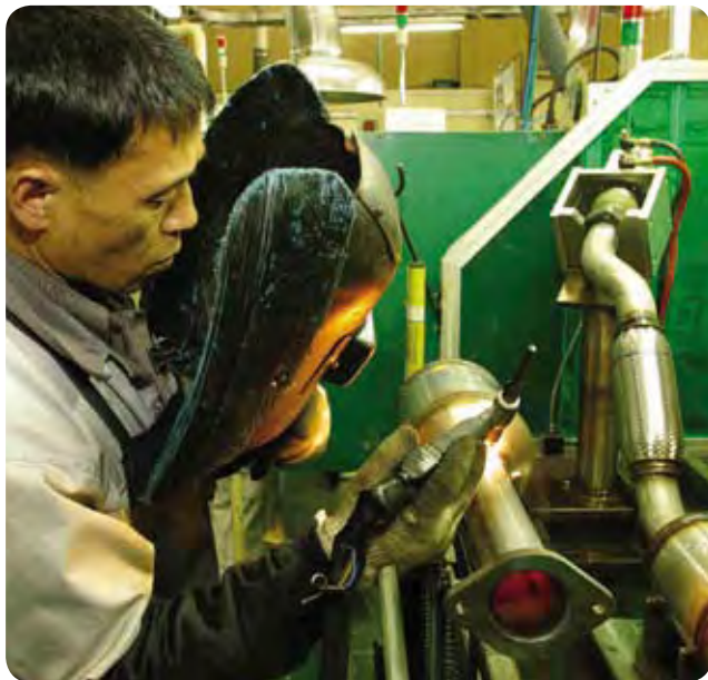
Exhaust system welding, grade 439, S. Korea.
