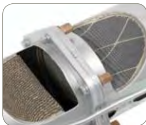
Grade 1.4509/441, diesel particle filter, Peugeot 607, Faurecia
