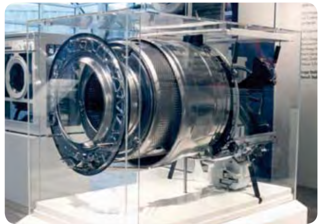
Exploded display of washing-machine interior.
