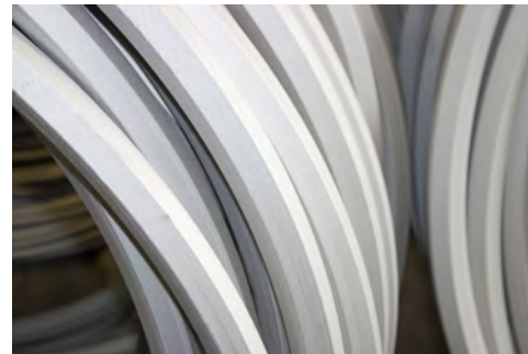
Hexagonal wire rod Ø14.5-31.5 mm
