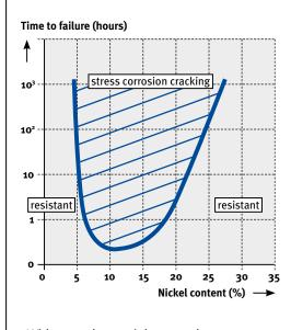
With regard to stainless steels, stress corrosion cracking only occurs in austenitic grades and is related to their nickel content. Steel grades with a nickel content in the range between 7 % and 15 % are all sus-
