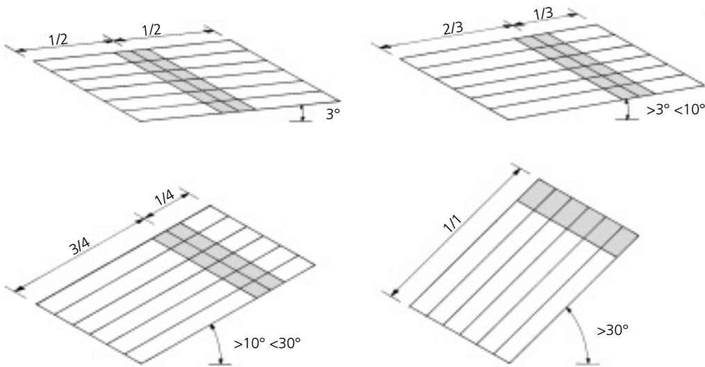
*The number and position of cleats depends on the pitch of the roof. Fixed cleats are positioned in the grey area.*
