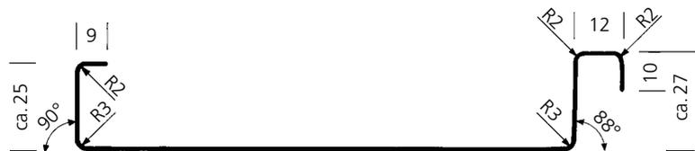
Typical section shape of a standing seam tray
