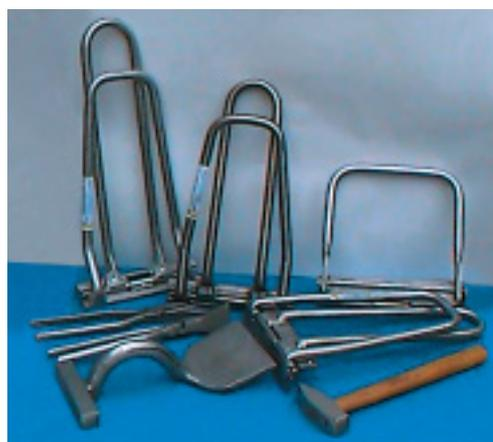
*Stainless steel roofs can be fabricated with the usual tools, provided contamination with carbon steel particles is prevented.*
