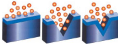
*Stainless steel builds up an invisible protective layer. If damaged, it re-forms spontaneously under the influence of oxygen from air or water.*
