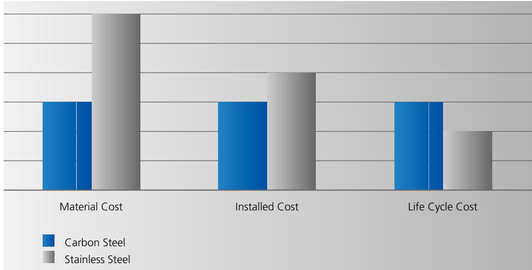
Cost comparison of 0.6 mm coated galvanised carbon steel and 0.4 mm stainless steel grade 1.4401: Due to the mechanical properties of stainless steels, the material thickness can be reduced to 0.5 or 0.4 mm, providing a lighter weight (3.2 kg/m<sup>2</sup> for 0.4 mm stainless steel as against 4.7 kg/m<sup>2</sup> for 0.7 mm coated carbon steel). While coated carbon steel has a life expectation of 15 to 20 years, the service life of a stainless steel roof is generally that of the building.
