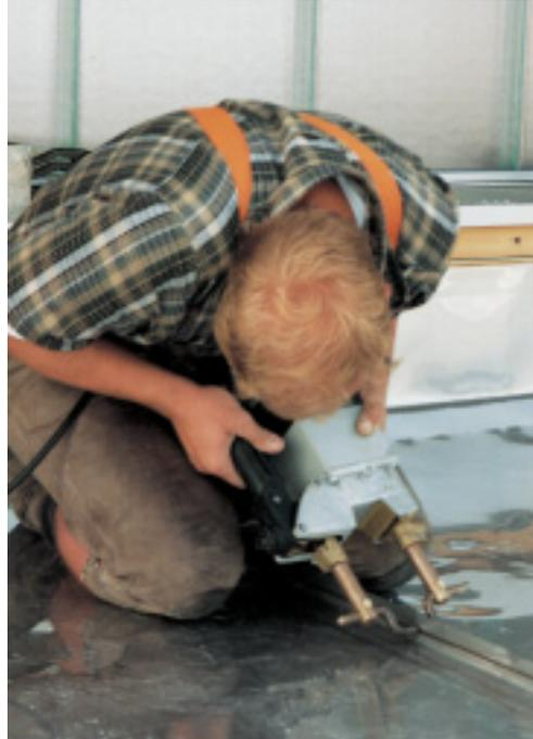
*Portable spot welding equipment*
