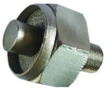
3D printed stainless steel pressure sensor
