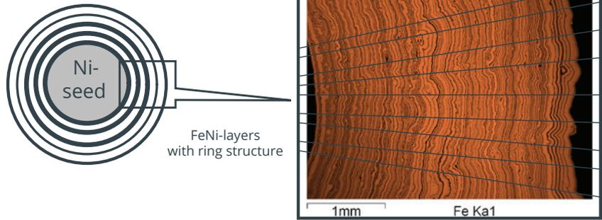
Figure 4 Layered structure of ferronickel pellets (dark color=Ni-rich, light color=iron-rich)
