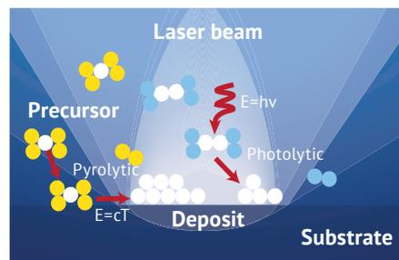
Figure 5 Laser beam guided selective area deposition from vapor phase metal precursor
