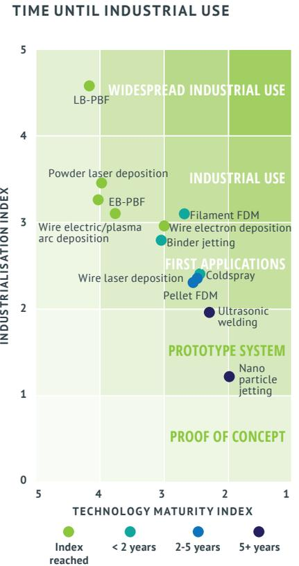
*Figure 2 Technology and industrial maturity index of different Metal AM technologies*
