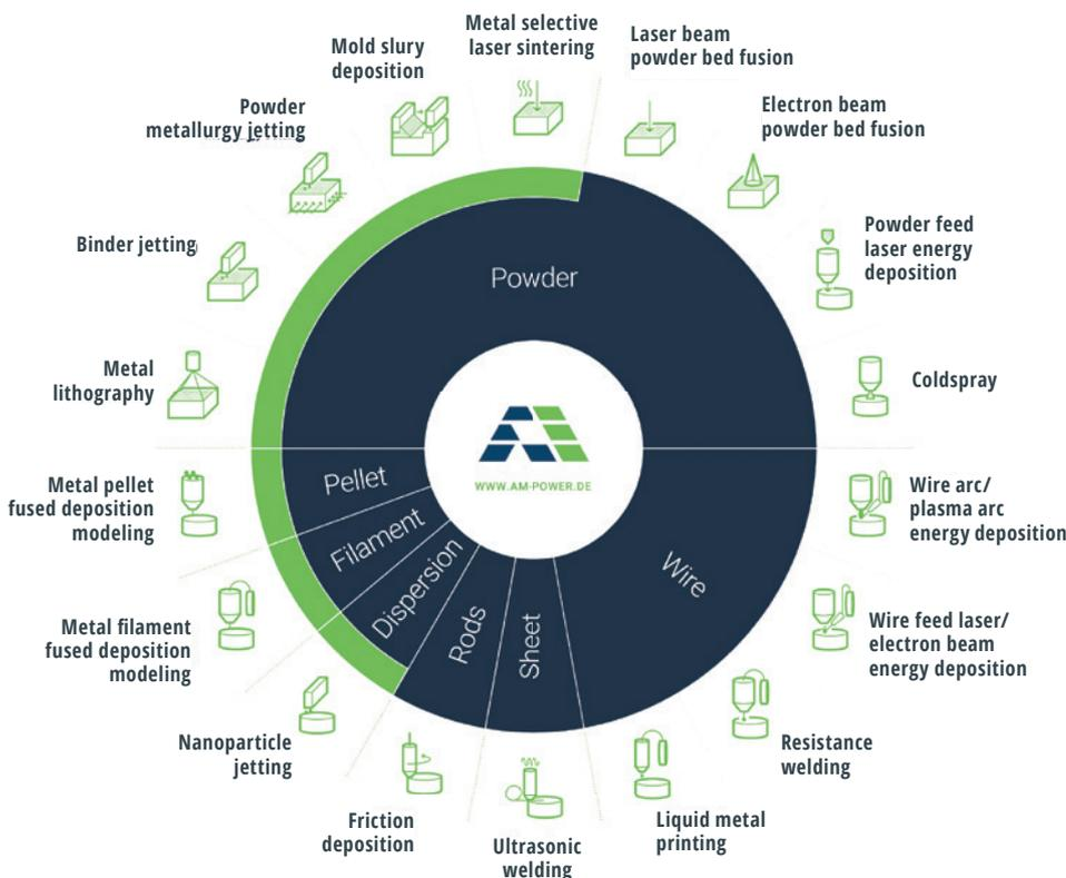
*Figure 3 Technology overview Metal Additive Manufacturing Over 18 different metal 3D printing processes are known. AMPOWER Insights provide an overview and classification of the most important procedures.*
