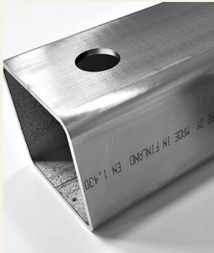
*Over four tonnes of stainless steel square and rectangular tubes in three sizes, from 0.5m to over 2m long, were supplied by Stalatube to fabricate the balcony frames. The grade of stainless steel chosen was Type 304 (UNS S30400). The tubes were laser cut and perforated to precise tolerances.*
