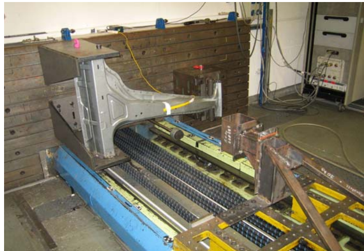
Figure 9. B-pillar for experimental crash-test
