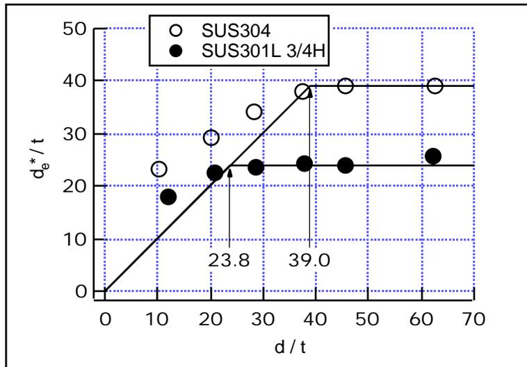
Figure 8 Effective width-to-thickness ratio of square box
