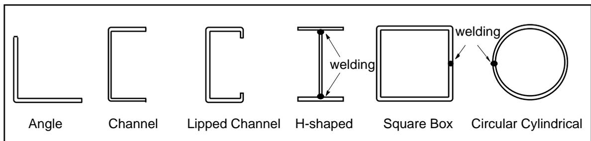
**Figure 2** Shapes of thin-walled stainless steel in the scope of the R & D program
