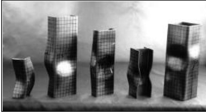
**Figure 4** Local buckling of thin-walled stainless steel stub-columns
