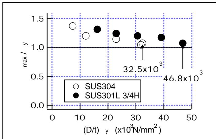
**Figure 11** Maximum compressive strength of circular cylinder
