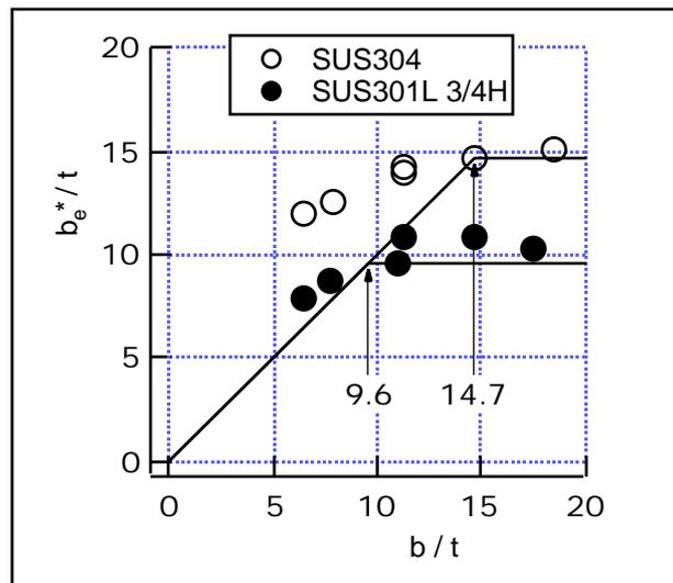
**Figure 7** Effective width-to-thickness ratio of angle
