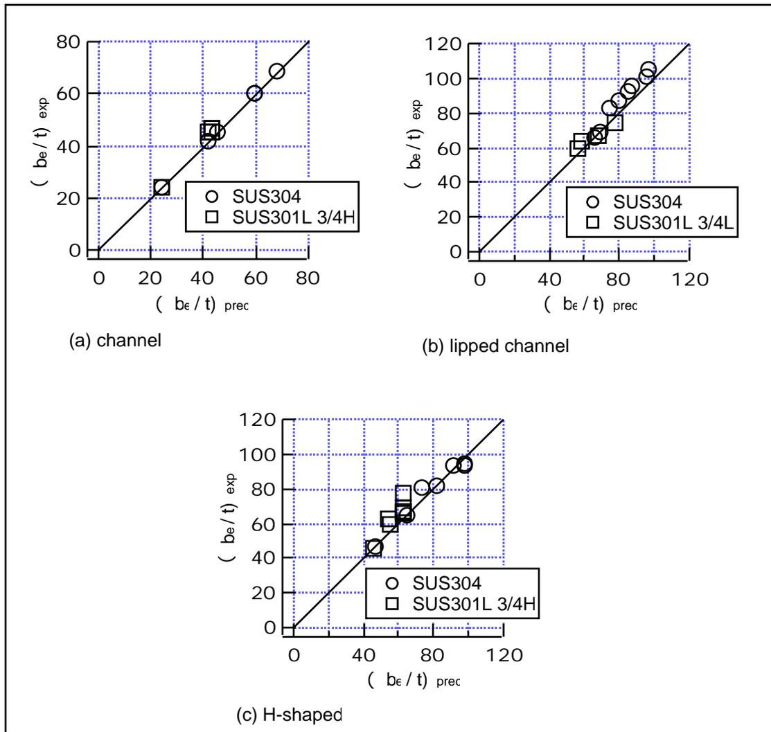
**Figure 9** Prediction vs. experiment of effective width-to-thickness ratio
