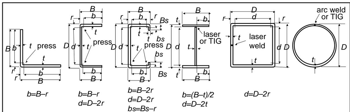
**Figure 3** Sections of stub-column specimens
