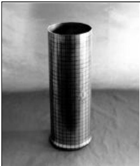
**Figure 10** Local buckling of thin-walled stainless steel cylindrical stub-columns
