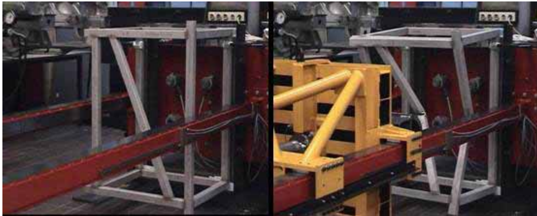
Figure 63. Frame before (left) and after (right) impact test (BUS p.169).
