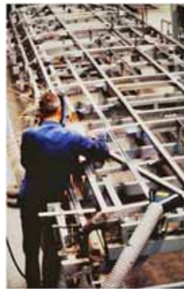
Figure 22. Welding of a bus chassis from square hollow sections, in grade EN 1.4301 (AISI 304) (Centro Inox 2007b).
