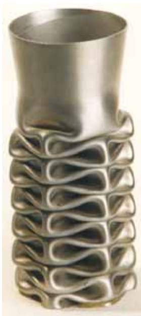
Figure 11. The crush behaviour of stainless steel circular hollow section maximises energy absorption in the event of a collision (Euro Inox 2006a).
