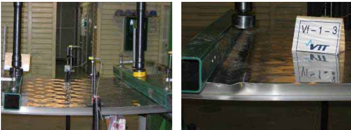
Figure 59. Details of panels in the four-point bending test, showing a) top-sheet wrinkling under compressive load and b) failure caused by local buckling of the core element.
