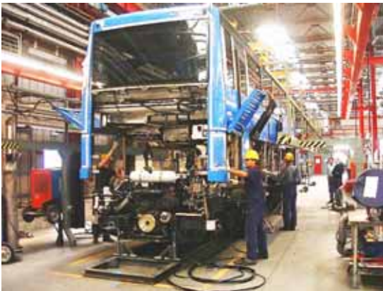
Figure 21. Assembly of buses with a stainless steel chassis and (ferritic) stainless steel skin (Centro Inox 2007a / De Simon 2007).
