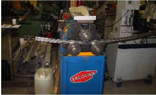
Figure 56. The three-roll tube-bending machine used in the DOLTRAC experiments.
