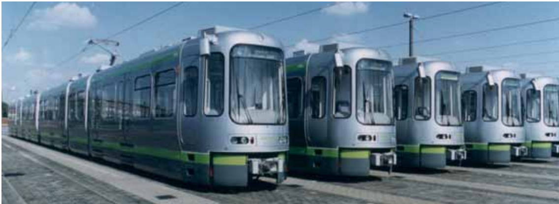
Figure 17. Trams in painted ferritic stainless steel, Hanover (Germany) (ThyssenKrupp Stainless 2007).
