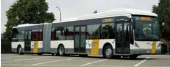
Figure 20. Articulated bus with a skin in ferritic stainless Steel (Van Hool 2007).
