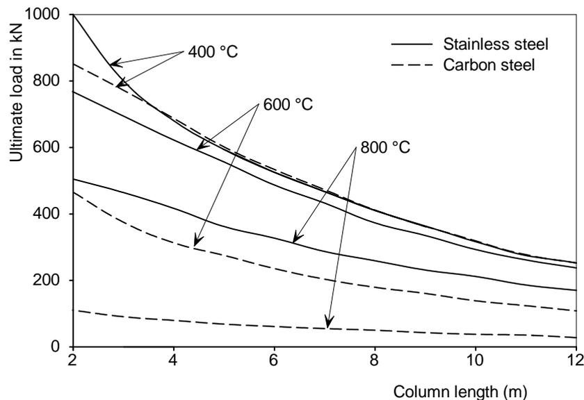
Figure 2. Ultimate loads for varying column length and cross-sectional temperatures
