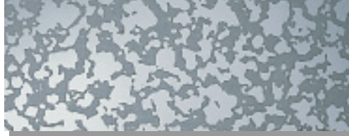
The depth of etching is controlled by the length of time that the stainless steel is exposed to the acid.
