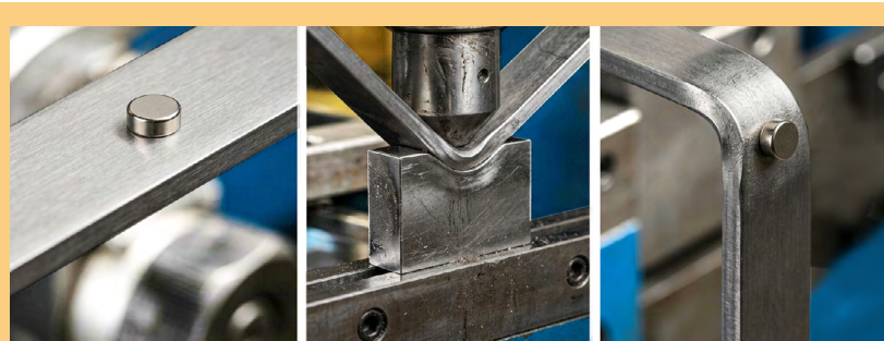
BEFORE 304 Stainless - Annealed, non magnetic
