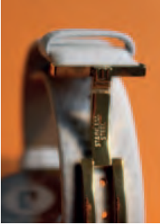
PVD coatings produce hard and scratch-resistant surfaces.
