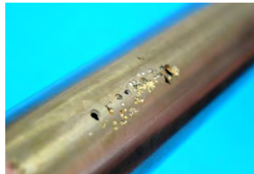
Concentrated bleach (chlorine) attack on 316 after a few weeks
