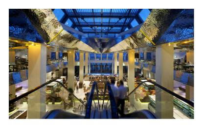
Perforated stainless steel panels help to absorb noise and add to the quality feel in this highend store.
