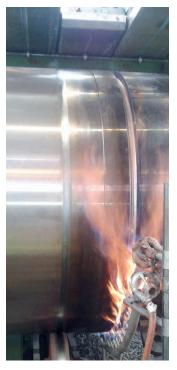
Figure 3. ENUN container body welding
