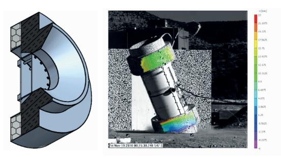
Figure 7. Detail of the impact limiter and drop test of the 1/3 scale model of the ENUN container
