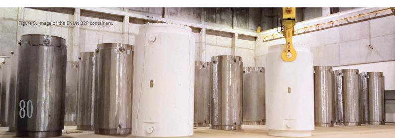
impact limiter, an additional protection that the cask carries in its transport mode.
