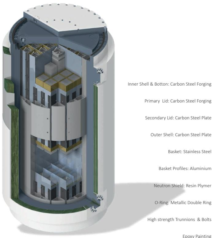
Figure 2. Main components of the ENUN cask
