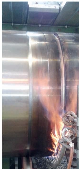
Figure 3. ENUN container body welding
