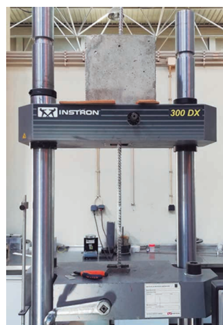
Figure 1. The pull-out test set-up
