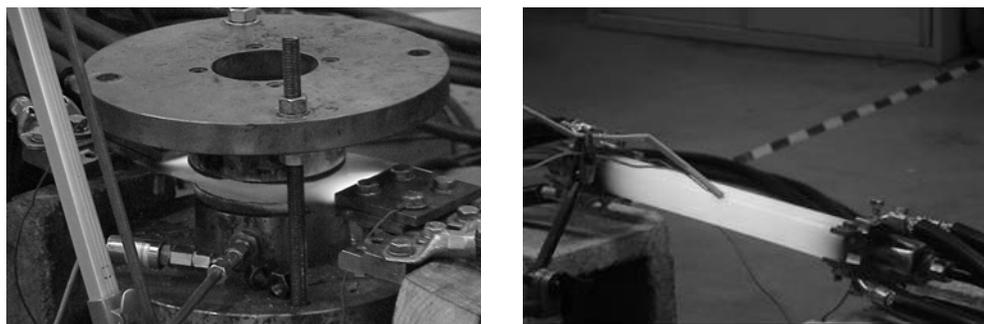
Figure 1. Experimental devices for the sheet (left) and tube (right) free expansion HMGF trials by LABEIN.
