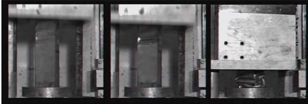
Figure 4. Crash process of a structured demonstrator from the beginning (left) to the end (right)
