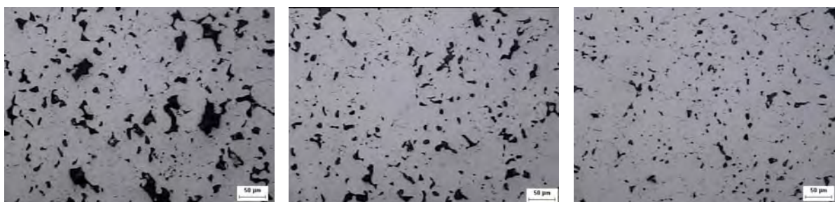
Figure 2. Cross sectional views of the three different PM stainless steels: ( left ) steel manufactured from 100% wa powder; ( centre ) steel manufactured from 90% wa powder + 10% ga powder; ( right ) steel manufactured from 80% wa powder + 20% ga powder
