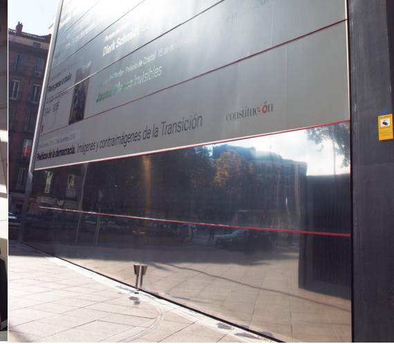
The Reina Sofia Museum, Madrid. Stainless steel plate glued to stainless steel plate with epoxy adhesive 3M™ Scotch-Weld 7260 B/A (year 2004)
