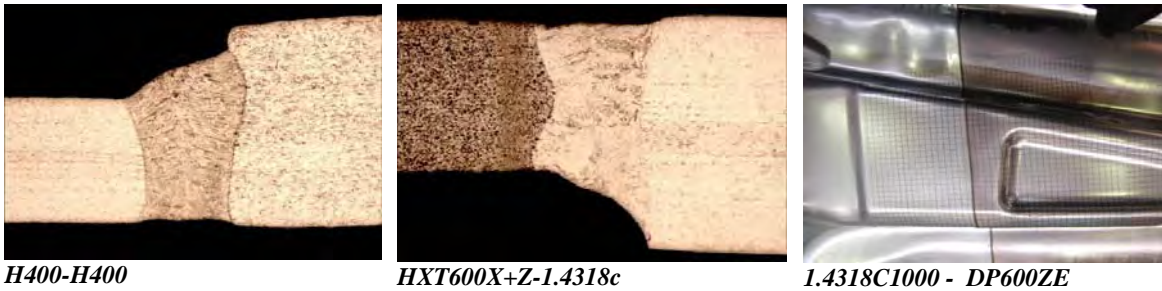
Figure 6. Microcraphs of stainless-stainless and mixed laser weld, tailor welded blank
