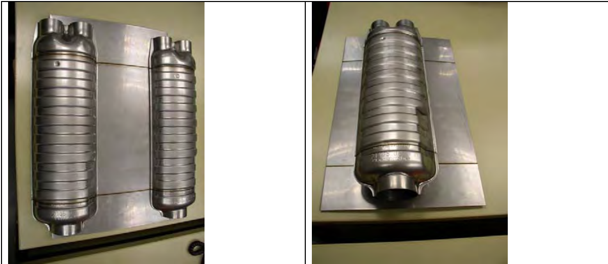
Figures 10 and 11. Exhaust system half shell in Grade 1.4301 before and after welding. Segments of 112 mm with t = 1.2 mm, 336 mm with t = 0.7 mm and 97 mm with t = 1.2 mm [2]
