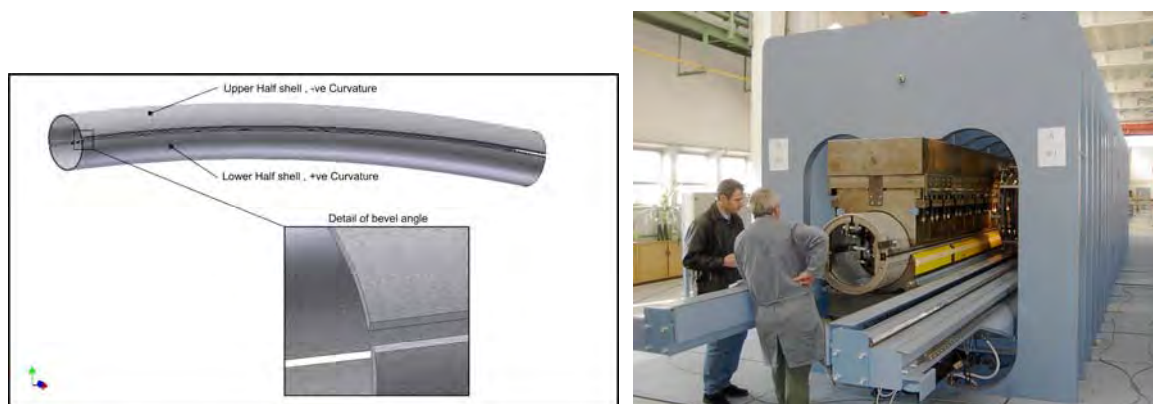
Figure 1. (a) schematic of half-shell curvature (not to scale), (b) a welding press at a Cold Mass Assembler
