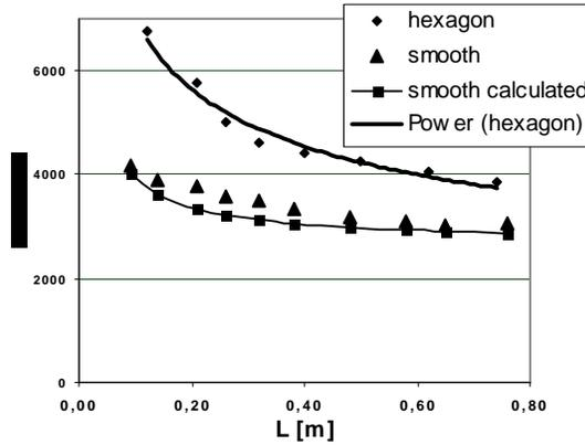
Figure 22. Convective heat transfer  $h$  versus the length of the conduit at Re number 30000 [11]
