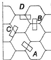
Figure 8. Cuttings of vault structured sample for material tests
