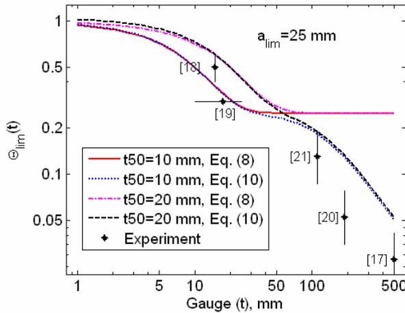
Figure 1. The functions  $\Theta_0(t)$  and  $\Theta_{lim}(t)$  ( $a_{lim} = 25$  mm) versus thickness  $t$  according Eqs. (8) and (10) for the  $t_{50}$  values 10 and 20 mm. Crack detection observations with their references are included.
