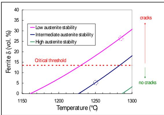
Figure 3. Evolution of delta ferrite content at hot rolling temperatures by ThermoCalc Software
