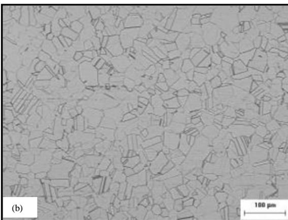
Figure 4 b). Typical austenitic microstructure of cold rolled strip for HNASS
