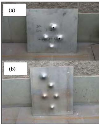
Figure 8. Samples of HNASS after ballistic test (b) according to EN1063 compared to 304 (a)
