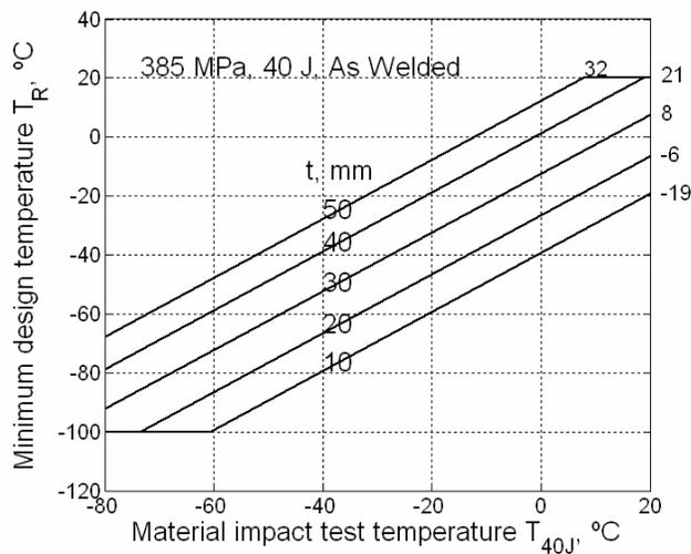
Figure 2. Model values for min design temperature  $T_R$  versus temperature where the Charpy impact toughness is 40 J. Values are given for wall thicknesses  $t$  between 10 and 50 mm. The yield strength is assumed to be 385 MPa, which corresponds to the values for DSS 2304.
