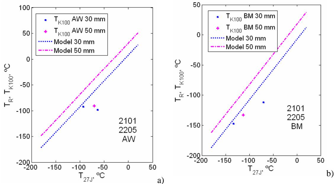
Figure 6. Measured  $T_{K100}$  and values for the minimum design reference temperature  $T_R$  as a function of the impact toughness specification temperature  $T_{27J}$ . Thicknesses 30 and 50 mm. The duplex stainless steels LDX 2101 and 2205.  $t_{50} = 10$  mm. a) As-welded (AW) condition. b) Base metal (BM).
