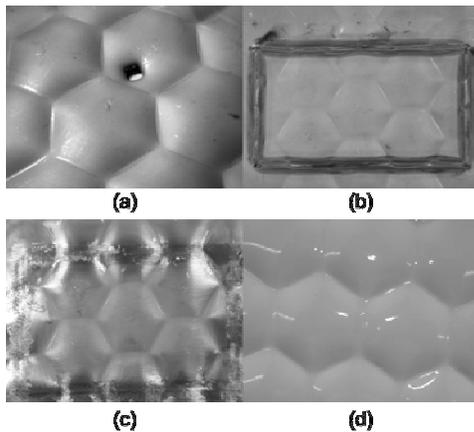
Figure 12. Welding tests using Cold Metal Transfer welding: (a) damaged vault-structured part, (b) substitution part welded in, (c) weldment joint after grinding, (d) repaired area after varnishing
