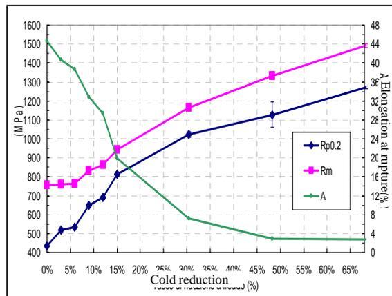
Fig. 5 The work hardening behaviour of AHNS
