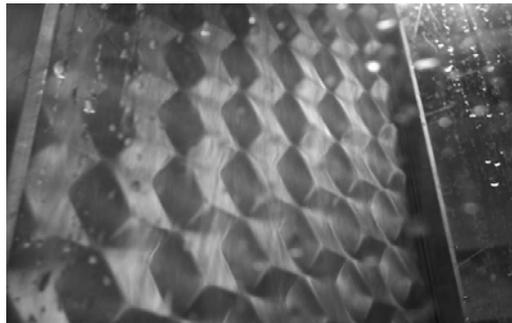
Figure 18. Thin film flowing across the faceted-structured sheet metal [10]
