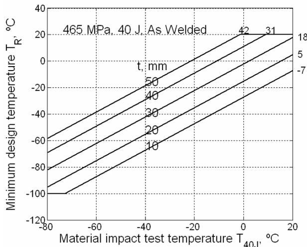
Figure 3. Same as Figure 2 for a yield strength of 460 MPa representing the DSS 2205 and LDX 2101
