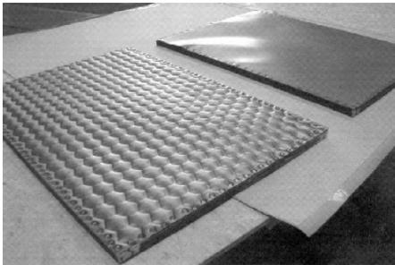
Figure 10. Vault-structured sheet metal of stainless steel spot welded on a frame
