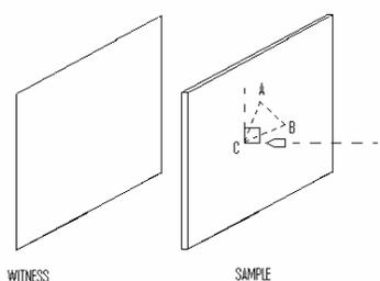
Impact test, for the evaluation of the ballistic behaviour, have been performed according to EN1063 standard that essentially prescribes speed and bullet type for the different qualification levels. Each sample (a 500  $\pm$ 5mm square plate) must be hit by 3 bullets whose impact points must form the vertex of a 120 mm side equilateral triangle and not release spalls, upon impact, on a thin paper sheet (witness) positioned behind (see figure on the left).
