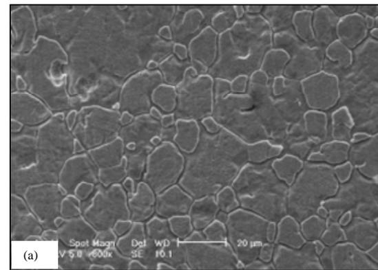
Figure 4 a). SEM micrograph of a cold pickled surface for HNASS
