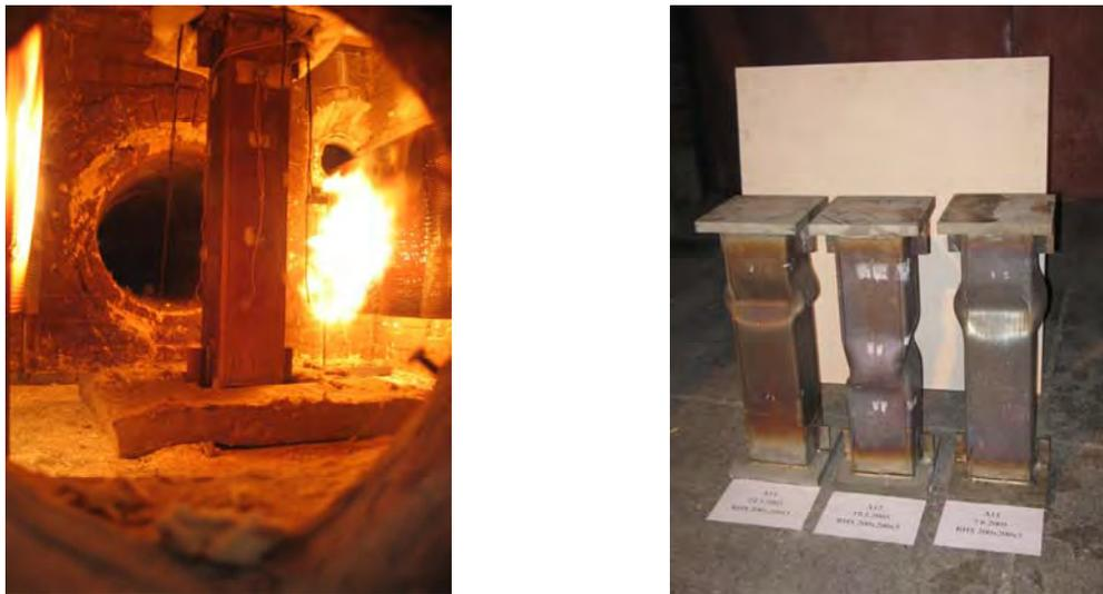
Figure 3. Tests on RHS with slender cross-sections
