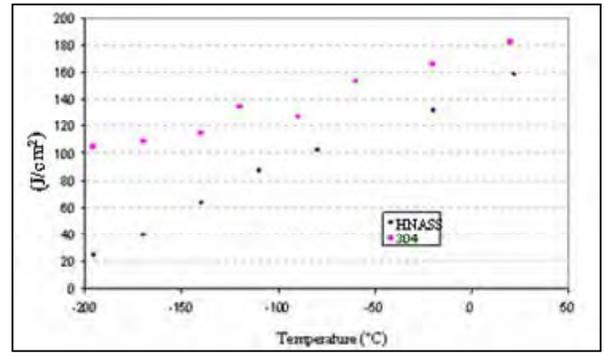
Figure 7. Charpy Impact energy of HNASS compared to 304 grade
