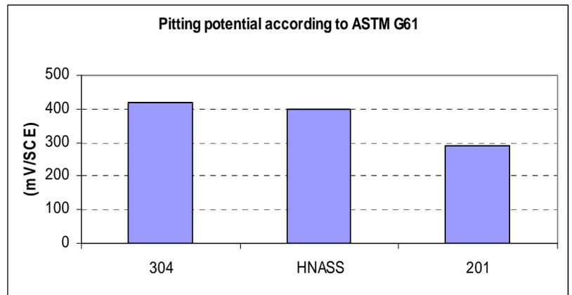
Figure 9. Corrosion resistance properties evaluated by pitting potential according to ASTM G61
