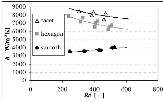
Figure 19. Largest local convective heat transfer coefficient  $h$  versus  $Re$  numbers [10]
