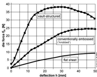
Figure 7. Flexural strength test of even, conventional embossed (“knobbed”) and vault-structured sheet metal using ductile steel FeP04
