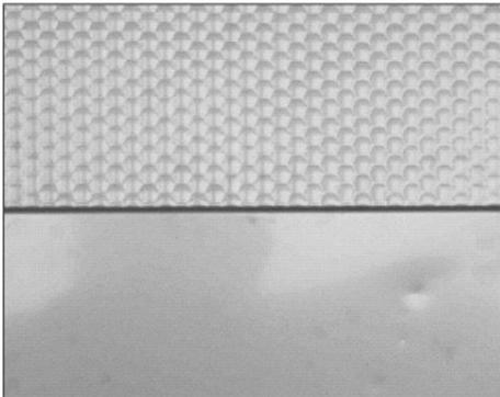
Figure 14. Comparison of unstructured and vault structured panel
