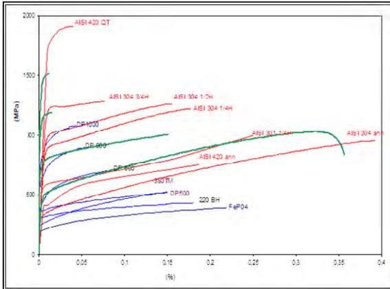
Figure 1. Mechanical strength and ductility of HNASS compared to other stainless steel grades
