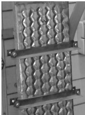
Figure 21. Conduit of vault-structured sheet metal of stainless steel [11]
