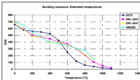
Figure 10. Buckling stress determined by anisothermal transient test according to EN 1993-1-2
