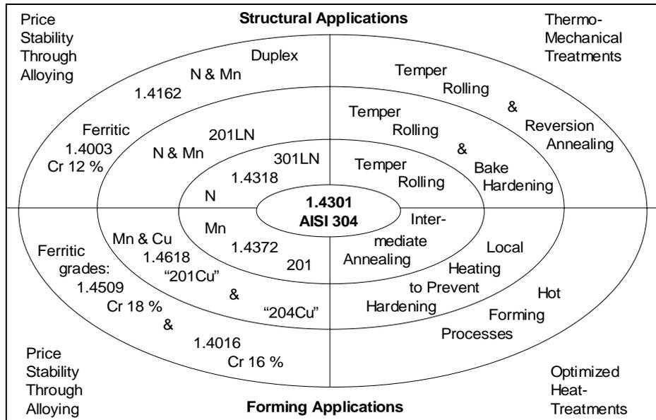
Figure 2. Optimising both material and manufacturing costs by using new alloys and novel treatments.
