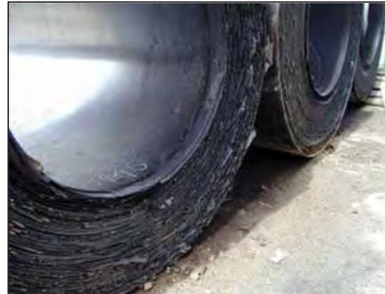
Figure 2. Edge crack on hot strip bands, due to high content of delta ferrite
