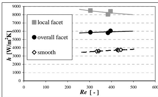
Figure 20. Local and average convective heat transfer coefficient  $h$  versus  $Re$  numbers [10]
