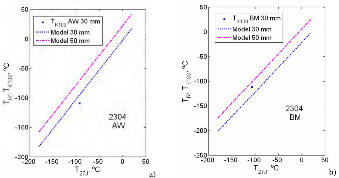
Figure 5. Measured  $T_{K100}$  and values for the minimum design reference temperature  $T_R$  as a function of the impact toughness specification temperature  $T_{27J}$ .  $T_{K100}$  is the temperature where the fracture toughness is  $K_{Jc} = 100 \text{ MPa}\sqrt{\text{m}}$ . Specimen thickness 30 mm. The duplex stainless steel 2304.  $t_{50} = 10 \text{ mm}$ . a) As-welded (AW) condition. b) Base metal (BM).
