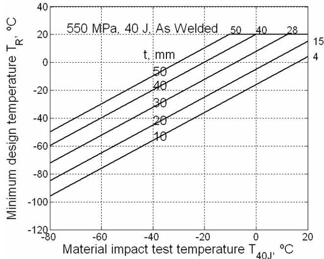
Figure 4. Same as for Figure 2 for a yield strength of 550 MPa representing the steel 2507
