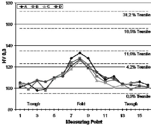
Figure 9. Vickers micro hardness values and tensile values (DX56D, SS 33mm)
