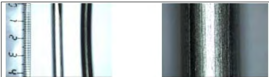
Figure 3. Photos of the Nikrothal 40 samples from continuous type hydrogen reduction
