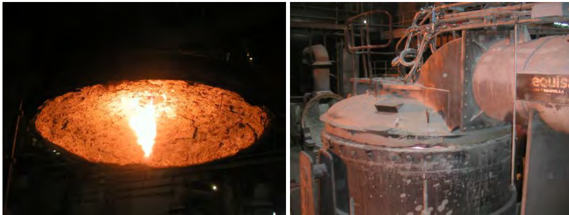
Figure 7. Ladle drying and preheating with flameless oxyfuel at Acerinox, Spain (fuel: natural gas).
