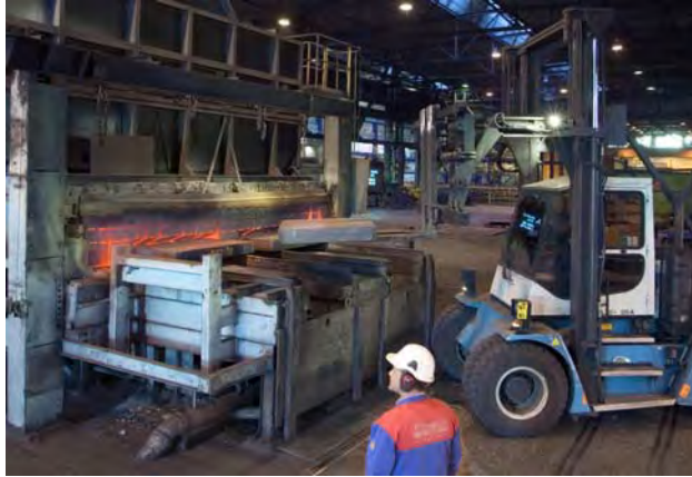
Figure 6. Outokumpu Stainless in Sweden increased their heating capacity in the existing walking beam furnace by 40-50% when implementing flameless oxyfuel (fuel: LPG). With this investment in an existing furnace plate mill could accumulate production volumes from another site.
