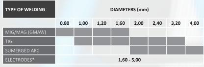
\*The material is supplied in wire coils or cut wire, subsequently coated before its final use
