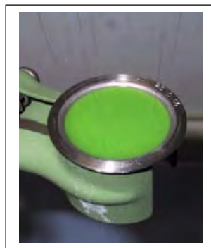
Figure 2. Deep-drawn stainless steel disk with microelectrodes embedded in resin
