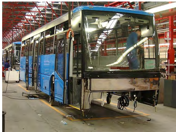
Figure 4 (above). Bus body in stainless steel (Source: Centro Inox / De Simon)
