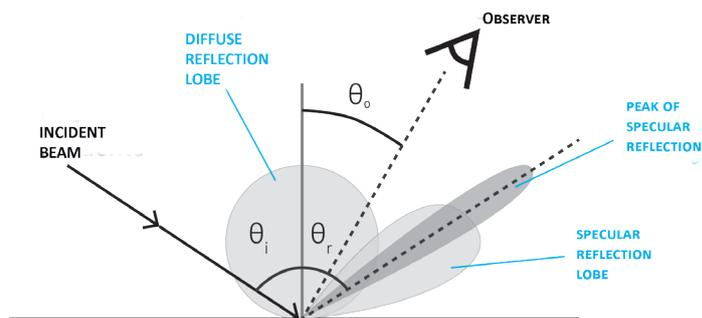
Figure 1: Illustrative diagram of the effect of roughness on the spatial distribution of the intensity of reflected light on a surface.
