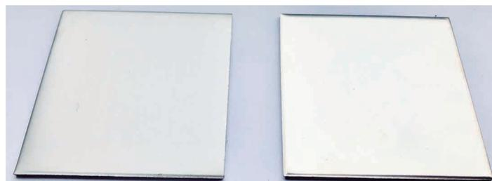
*Stainless steel test samples supplied by ACERINOX, S.A. : Left. 01VSAP (finish 2B) with LRV (di) 57,868 and (de) 55,450; Right 03V3MCB (Finish BA) with LRV (di) 56,384 and (de) 10,521.*
