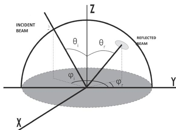
Figure 2: Illustration of the reference frame used for the measurement of bidirectional reflectance.
